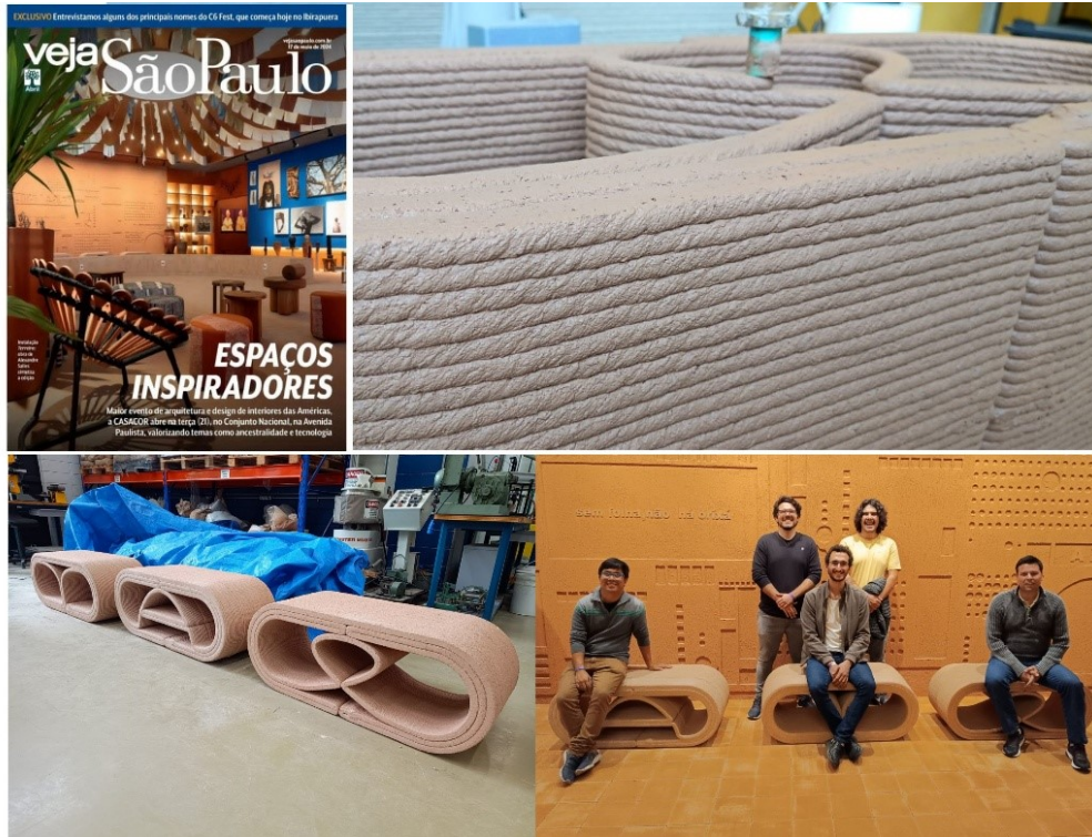
Figure 4. AYE benches exhibited at Casacor 2024, Latin America’s largest architecture, landscaping, and interior design exhibition (bottom right). The top right image shows the 3D printing process of one of the benches, highlighting the layered manufacturing technique. The top left features the exhibition’s recognition on the cover of a prominent Brazilian magazine. The bottom left image captures the benches after the production phase at hubic, developed by the Portal 3D team, prior to installation at the exhibition.
