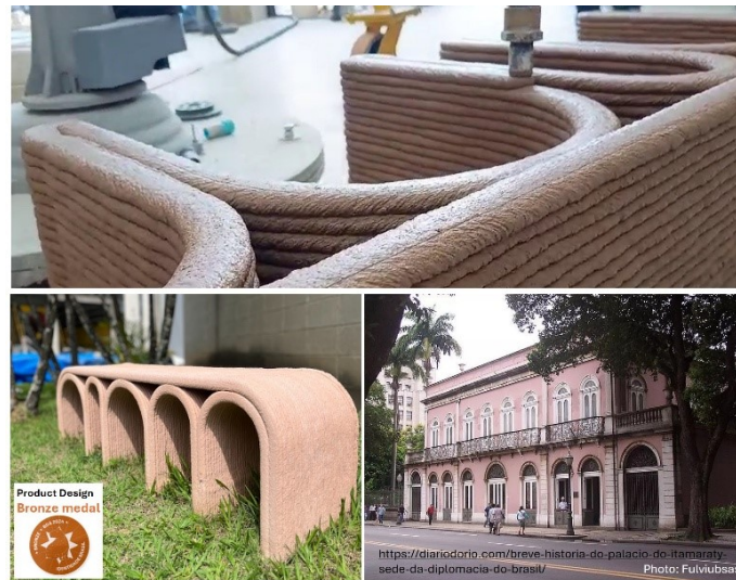
Figure 2. “Itamaraty Bench”, developed by Studio Manga_be Architecture and Design. The top image shows the bench during the 3D printing process using a bauxite residue-based cementitious formulation. On the bottom left, the final piece is displayed in an outdoor setting, highlighting its distinctive asymmetric arches. On the bottom right, the façade of the historic Palacete-Cor-de-Rosa of Marchioness of Itamaraty, located in Rio de Janeiro, is presented (the architectural reference that inspired the designer).
